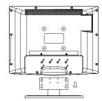
3.Use the four screws provided to fix the TV onto a wall mounting bracket via the 4 VESA standard holes on the back of the television.
